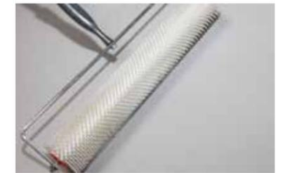
14. Immediately after smoothing the material should be de-aired with a spiked roller. Spiked shoes must be worn during application while walking over the fresh material.
